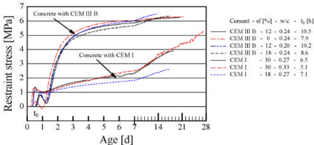
Figure 7: Centric tensile stress due to restrained autogenous deformation
