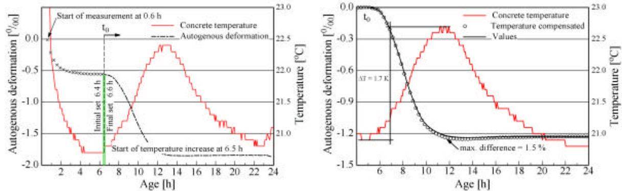
Figure 4: (left) Comparison of autogenous deformation, temperature development and setting (Vicat needle test); (right) effect of hydration heat on measured deformation
